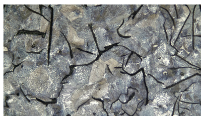
Grey Cast iron (objective: 50X)
