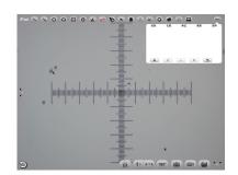
Step 4: Enter the name, the actual length of the calibration scale, and select the unit. When you draw on the ruler, the pixels are automatically entered as shown below. Click "OK" to complete the calibration;
