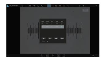
The lower part of the calibration table supports re-editing and deleting the selected calibration values.
