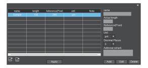
Step 3: When using the mouse to draw a straight line on the micrometer image and setting the scale length, selecting a longer scale length will give more accurate results. For example, selecting 10 small scale lengths will give you more accuracy than selecting only 1 scale length. After releasing the mouse, the image value of the line drawn with the mouse will be automatically updated in the "Benchmark" of the calibration table, as shown in the following figure:
